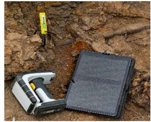
Hardware used: TSL RFID Reader, HID zip-tie RFID tag and ruggedized iPad loaded with InfraMarker RFID middleware and Esri's Survey123 data collection software.
